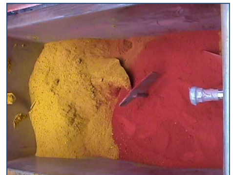
Ingredient before mixing - consisting of colour, hardener, and aggregate, particles 600-2000 um.
