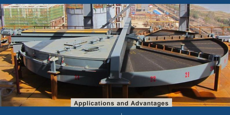
CPE pan vacuum filters are suitable for continuous filtration of rapid settling, free filtering solids and are designed for ease of installation, reliable operation, rapid dewatering, and efficient cake washing at large capacities.
