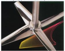
The critical performance measurement is the agitator flow rate.
