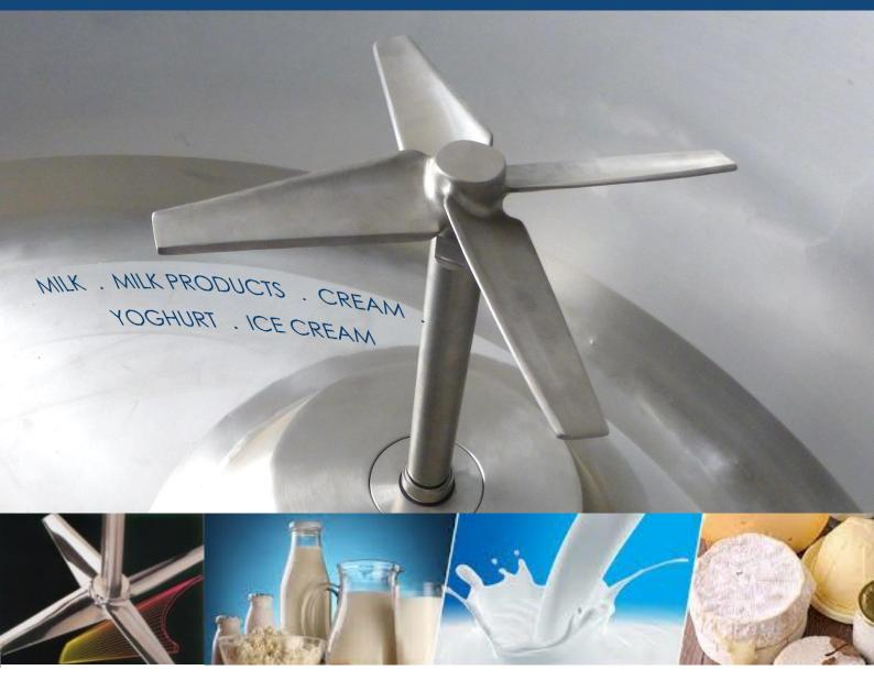
Chemical Plant & Engineering designs and manufactures the high efficiency RTF4 agitator suitable for dairy processing applications.
