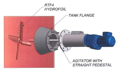
The location of the agitator in the tank should be as per the following drawings.
