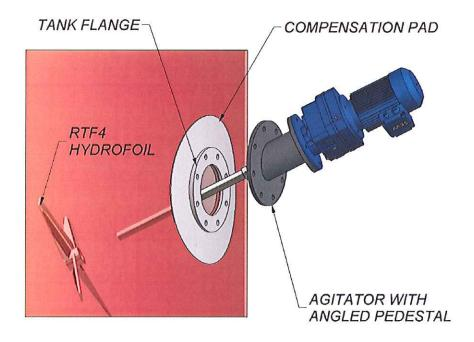
The location of the agitator in the tank should be as per the following drawings.
