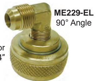
Enables the installation of a 1/4" MNPT hydrostatic relief valve in a safe, protected area. This two piece carburetion hose fitting fits all stainless steel braided LP-Gas hose with a 5/16" ID. The tank valve side has a 3/8" female flare and zinc plated for maximum corrosion resistance.
