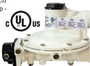
**MEGR-1632E Full Size Series:** Offers all of the same features as the compact MEGR-1232E series in a full size high capacity version. The full size MEGR-1632E diaphragm provides superior downstream regulation, has heavy duty wrench flats and a large 3/4" FNPT tapped drip lip vent to help prevent relief vent blockage.
