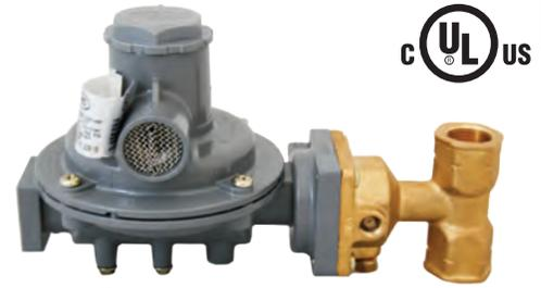
**MEGR-1232T Compact Series:** Offers a compact integral two-stage regulator design perfect for lower BTU applications and confined spaces. They feature an adjustment range from 9-13" WC (factory set @ 11" WC). Stainless steel integral components, fluorocarbon (FKM) seat discs, molded lip fabric reinforced diaphragms, and large precision machined aluminum orifices providing superior downstream regulation and maximum corrosion resistance against weather or contaminated gas.
