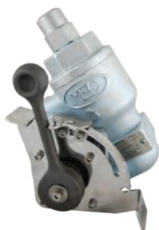
**Normal Bypass Mode:** functions just like our standard ME840 Series bypass valve during domestic tank deliveries by pushing maximum pump output to the hose end delivery nozzle while protecting the pump if the nozzle is closed during delivery.
