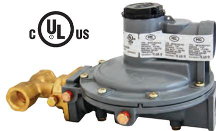
**MEGR-1632T Full Size Series:** Offers all of the same features as the compact MEGR-1232 series in a full size high capacity version. The full size MEGR-1632 diaphragm provides superior downstream regulation, has heavy duty wrench flats and a large 3/4" FNPT tapped drip lip vent to help prevent relief vent blockage.
