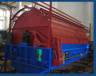
CPE drum vacuum filters consist essentially of a cloth covered drum rotating in a tank filled with the slurry to be filtered.
