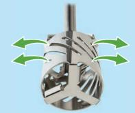
4. The high velocity radially discharged streams impact the slower moving tank flow for additional hydrodynamic shear and circulation, thus ensuring high flow, with no dead spots in the mix tank.
