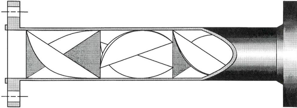
The Chemplant Static Mixer is an inline mixing device with no moving parts. This makes it a unique piece of processing equipment as it requires no external power source and is completely maintenance free. The Chemplant Static Mixer produces a homogeneous blend or dispersion in a laminar, transitional or turbulent flow regime within a very short length of pipe.
